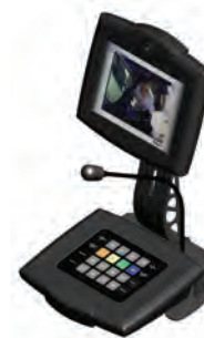
CCS-1561 Optional Audio/ Video Station for 1 to 16 lanes provides exceptionally clear audio and video with a high contrast 6.4" color LCD Monitor.
